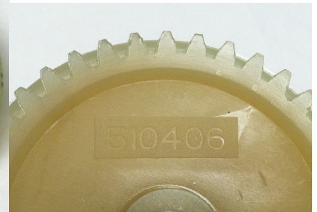
Figure 4. K3008 Distributor Gear Marked 510406 (Backside)
